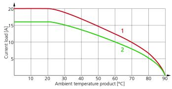
1: Base curve 2: Derived curve according to DIN 60512-5-2 with correction factor 0,8
